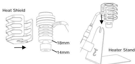
Install heat shield fully onto nail stem above the joint section. Use CAUTION not to bend the heater neck.
