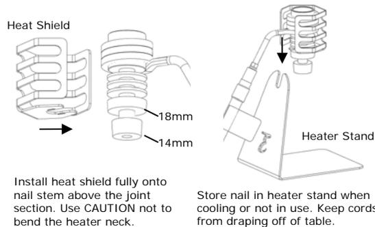
Install heat shield fully onto nail stem above the joint section. Use CAUTION not to bend the heater neck.
